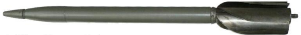
Type 4: six rolled up (less stiff) steel fins with a rounded nose.
