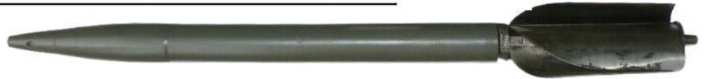
Type 1: four rolled up (very stiff) steel fins with a rounded nose, resembles type 3 with three fins.
