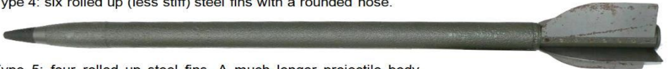
Type 5: four rolled up steel fins. A much longer projectile body.
